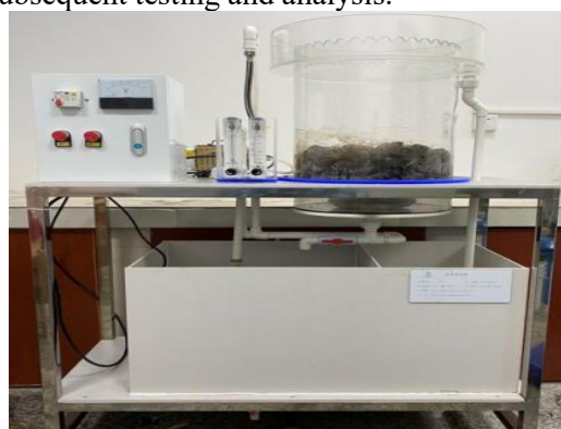
Figure 5. Iron-carbon Micro-electrolysis Treatment Device
