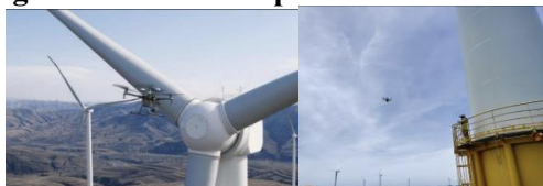
Figure 3. UAV Inspection of Wind Turbine Blades
