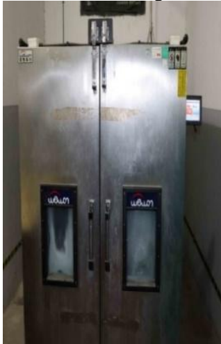
Figure 1. High-Temperature Safety Test for 48mm OC Tear Gas Grenade Packaging
