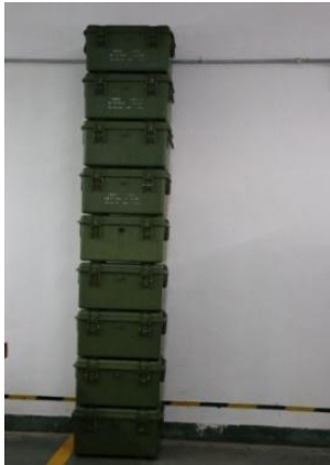
Figure 2. Stacking Safety Test for 48mm OC Tear Gas Grenade Packaging
