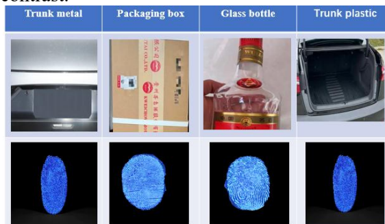
Figure 6. Latent Fingerprint Images on Different Object Surfaces Revealed by N-CQDs@MMT (365 nm, UV)
