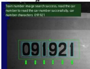
**Figure 9. STrain Number Identification Test Effect.**
