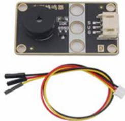
Figure 6. Warning Output Module
