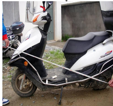
Figure 8. Relationship between the Left Front Guard-Panel Trace and the Left Rear Foot-Peg Trace
