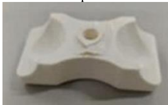
Figure 11. Broken Hinge Block
